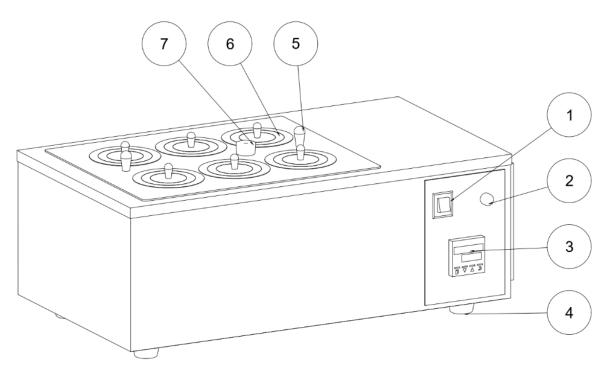
Figure 1: Component Diagram of Water Bath with 6 holes
